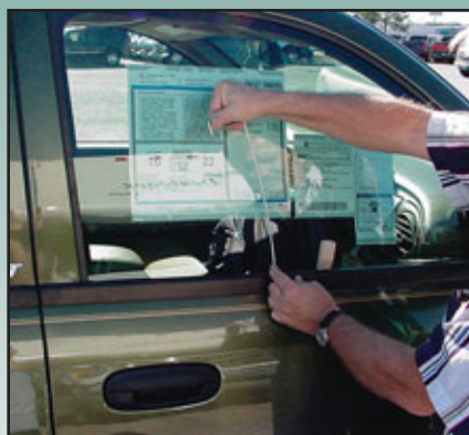
9. Twist the tool and lever the linkage rod forward to unlock.
